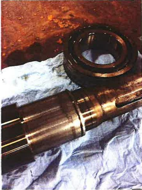
Outboard bearing shaft fit is ok.
