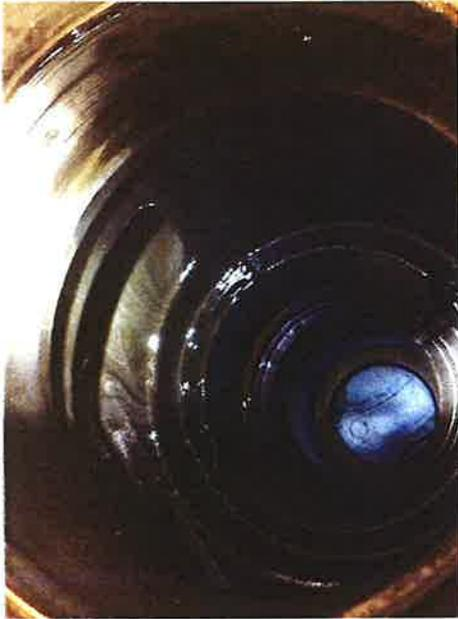
Metal particles, and sludge in the bearing oil.
