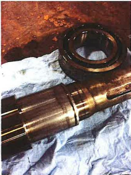
Shaft is ok at the bearing fit for the inboard bearing
