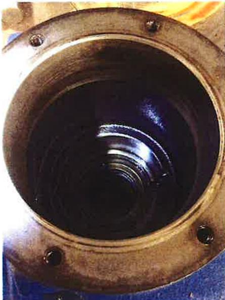
Inboard bearing had spun in the bearing housing.
