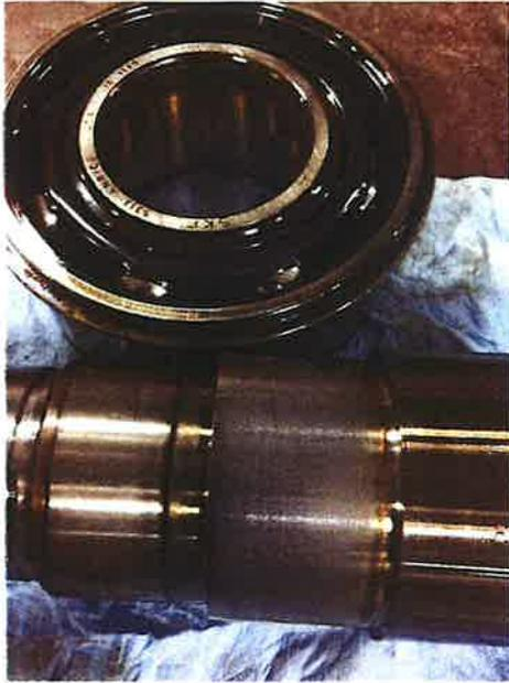
Shaft is ok at the bearing fits on outboard bearing.
