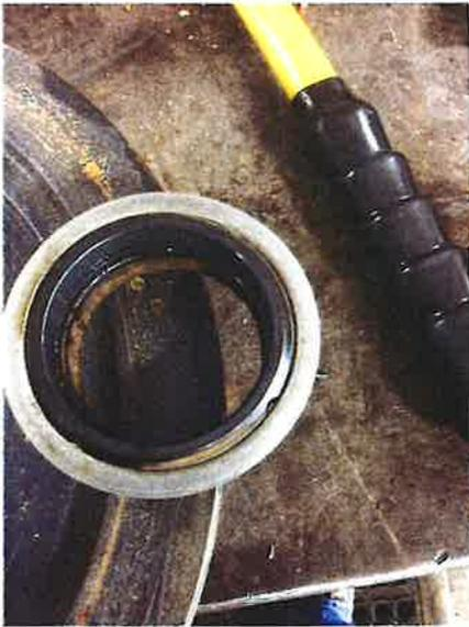
Rotating element for the mechanical seal is bad,
